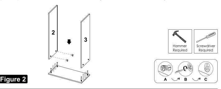
Step 3 : Fix Minifixs & Dowels on Board 2 & 3 as shown in Figure 3. Tilt Board 2 & 3 a little to fix Board 4 & 5 between Board 2 & 3. Fasten the Minifix Housings as shown in figure below.
